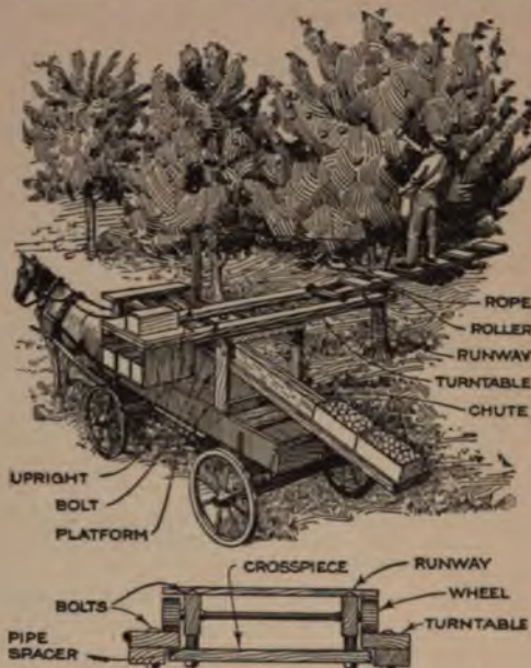
DETAIL OF RUNWAY LOCKING ARRANGEMENT
